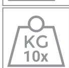
When suspending the fixture above ground level, verify that the structure can hold at least 10 times the weight of all installed devices. Use the safety cable to secure the fixture in addition to the primary mounting bracket.
