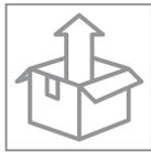
**2. Unpack the VirtuaLine™ LED SWITCH and power supply:** Carefully remove the projector from the box and inspect it for any physical damage which may have occurred during shipping, then do the same for the power supply and relay box. If any physical damage or moisture is present, contact Laserglow immediately to report it.
