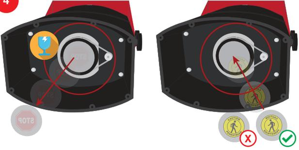
Carefully remove the old image template and replace it with the new image template. The image template should appear to be backwards or mirrored when looking into the front of the projector.
