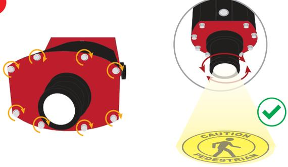
Replace the front cover and adjust the focus as needed. You will likely need to use the image rotator to align the projection as well.
