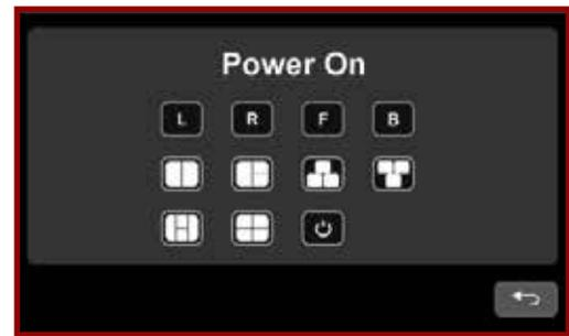
The "Power On" settings allow the start up mode of the system to be changed. Changing this setting will change what is displayed on the screen after the system is power cycled. The 7" options are shown on the right and the 10.1" options are shown on the left.
