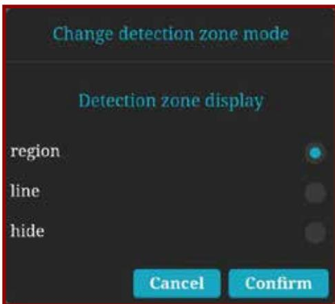
Detection zone display changes the style of the detection zones on the display for each camera. "Region" shows the red, yellow and green zones while "Line" shows just lines for bounding each region. Selecting "Hide" removes all of the regions or lines from the display.
