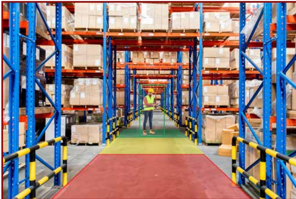
If a pedestrian is detected in multiple zones, the audible signal is that of the highest priority zone. For example if a pedestrian is detected in the green zone and red zone, the red zone signal will alert the driver.
