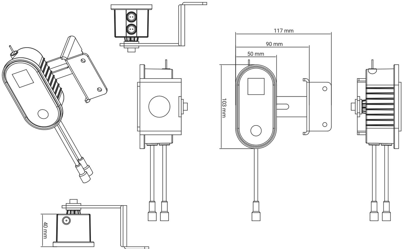
Mount the bracket to the center of the forklift carriage, aligning so that the laser module is approximately level with the top of the forklift's tines.
